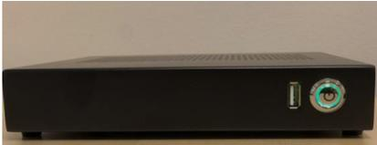
2. Press and hold the button on the front of the device for 5-10 seconds. The device will recycle, and the light should turn green.
